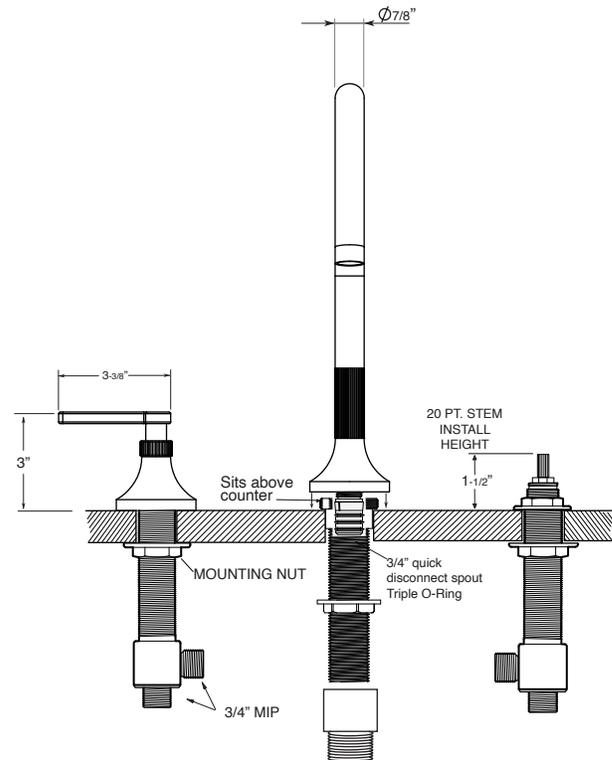
Spout and valves install through 1-1/4" diameter holes.
